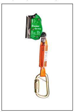
with an inline integral energy absorber that maintains an Average Arrest Force of less than 1,350 lbs. and a Maximum Arrest Force of under 1,800 lbs. The twist lock steel captive eye carabiner, serves as a convenient connection point and maintains the 12" or less (cable to sternal D-ring),
