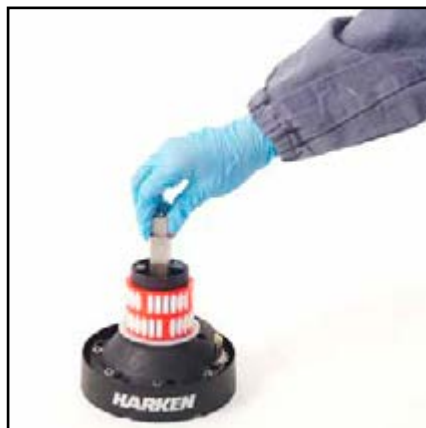
8. Slide out the central shaft n°19
