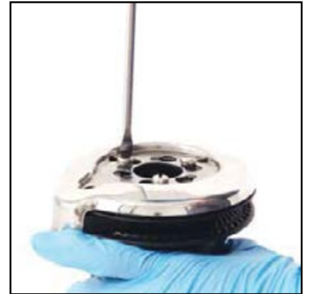
3. Unscrew the three screws n°27 (4 Nm/35 in-lb)
