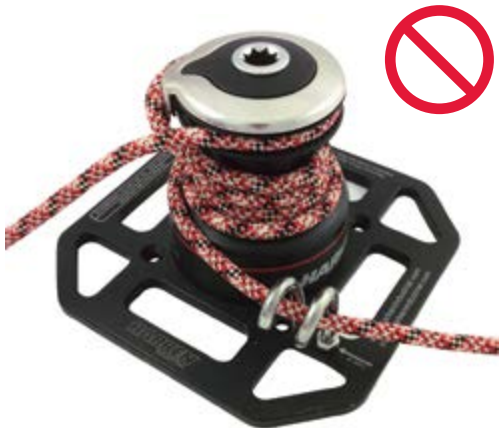
Excessive turns at base of winch
