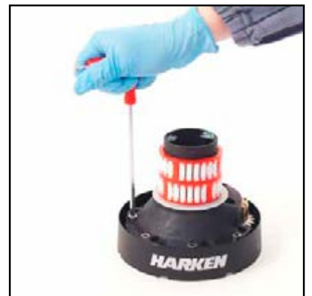
9. Unscrew the 6 stainless hex screws n°16 (8 Nm/71 in-lb) NOTE not those painted red
