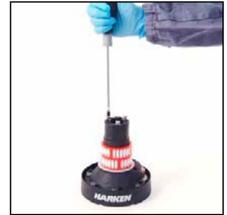
6. Completely unscrew three screws n°27
