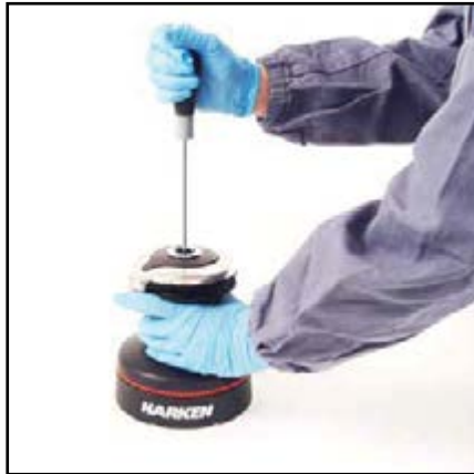
1. Unscrew the central screw (2 Nm/18 in-lb)
