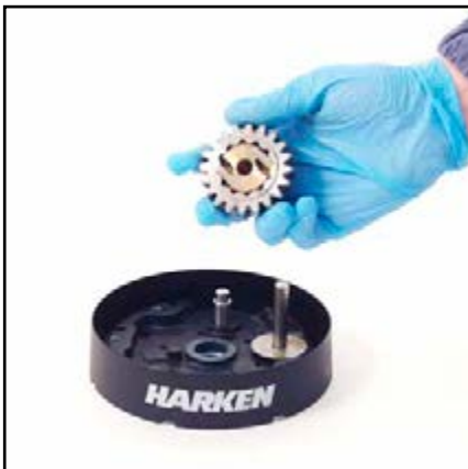
17. Remove the pawls n°5. To facilitate the operation press the spring against the pawl with a blade.
