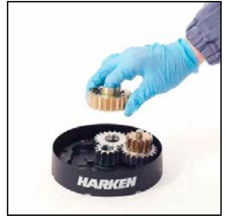
13. Remove the gear n°7 and remove the pawls n°5. To facilitate the operation press the spring against the pawl with a blade.
