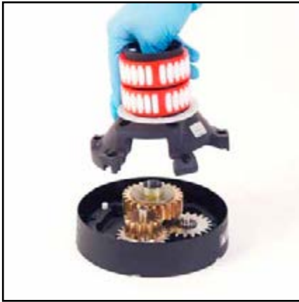
11. Remove the drum support n°15 Important: washer n°12 may remain inside the drum support!
