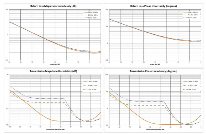
Full 1-path, 2-port forward path calibration with isolation, high power, 10 Hz IFBW, no averaging, 10 minute warm-up. OSLN50A-8, OSLNF50A-8, TOSLN50A-8, or TOSLNF50A-8 calibration kit. Reflection and Transmission Tracking are typical.
