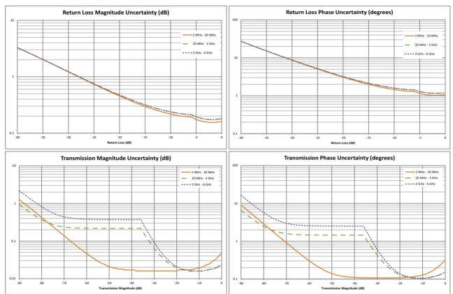
Full 1-path, 2-port forward path calibration with isolation, high power, 10 Hz IFBW, no averaging, 10 minute warm-up. TOSLK50A-20, TOSLKF50A-20 calibration kit. Reflection and Transmission Tracking are typical.
